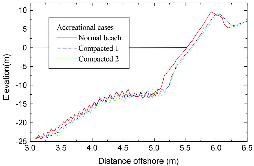
Fig. 6 Accretional profiles with different compaction.
