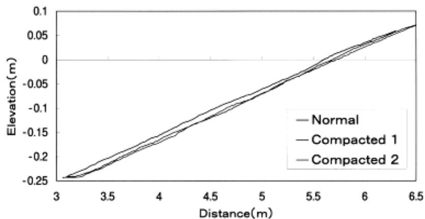
Fig. 3. Initial beach profiles with different level of compaction.
