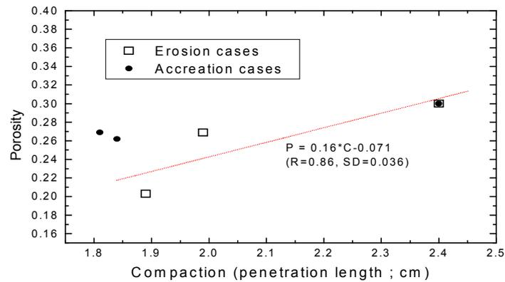
Fig. 9 A relationship between average compaction and mean porosity.
