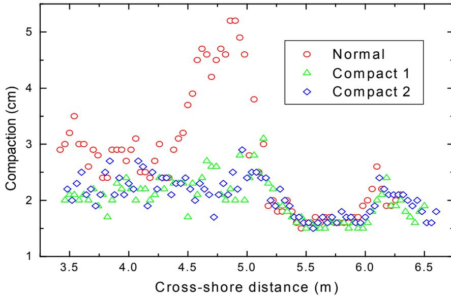
Fig. 8. Compaction distribution over berm profiles.
