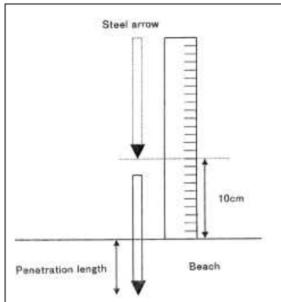
Fig. 4. Measuring techniques of compaction.
