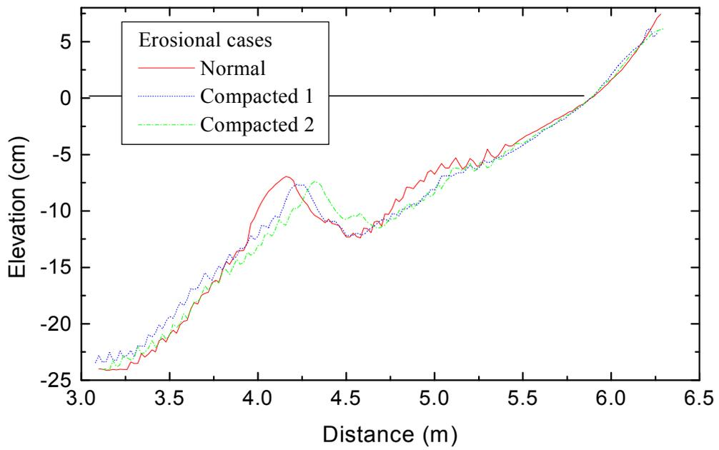
Fig. 5 Erosional profiles with different degrees of compaction.
