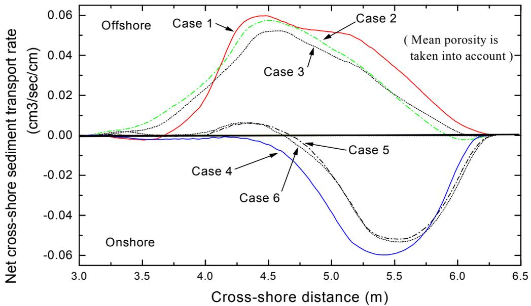
Fig. 11. Net cross-shore sediment transport rate estimated with average porosity.
