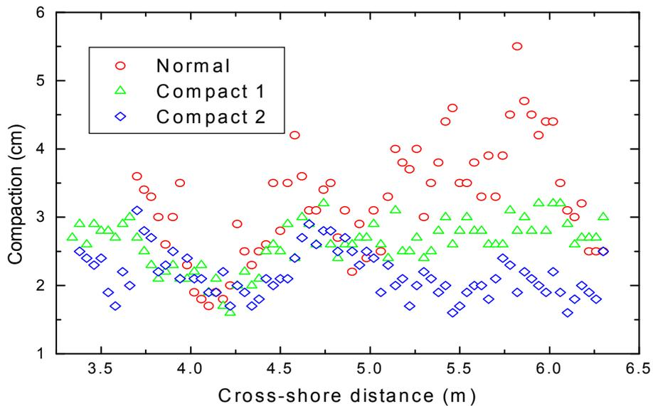
Fig. 7. Compaction distribution over bar profiles.
