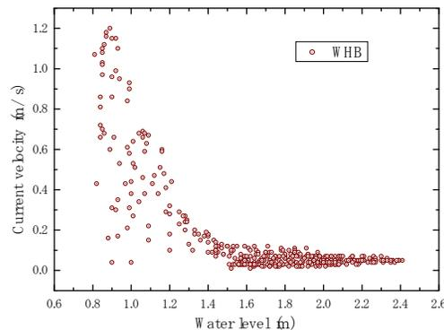
Figure 8. Relationship between current velocity and water level
